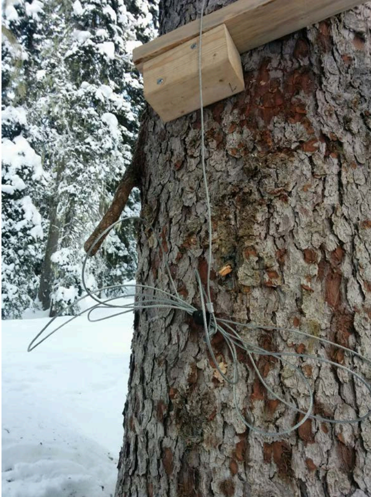
Figure 3 Lower attachment point for the wire spanned between trees. The tail is long enough to allow lowering of wire during re-baiting of the camera stations. Ten camera stations were deployed as part of the pilot field season in winter 2017, in the Columbia Mountains, BC.
