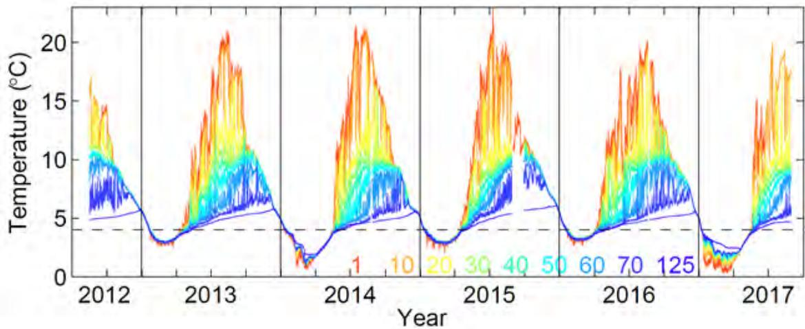
Figure 15. Temperature at selected depths at Revelstoke Forebay, 2012-2017. The dash line marks 4 °C, the temperature of maximum density. Depth is indicated by colour gradient.
