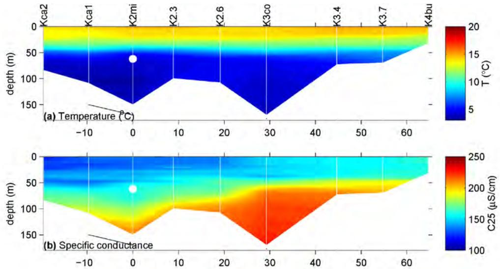
Figure 13. (a) Temperature and (b) conductivity in Kinbasket Reservoir, 15-17 September 2008. The outlet is marked at 62 m with a circle. White lines mark the location of the CTD casts. The contour is taken along the length of Canoe and Columbia Reaches, where Kca1 is the Canoe sampling station, K2mi is in the main pool, K3co is the Columbia sampling station in Old Kinbasket Lake, and k4bu is in Bush Pool (Figure 1, see Pieters and Lawrence 2018c for detail).
