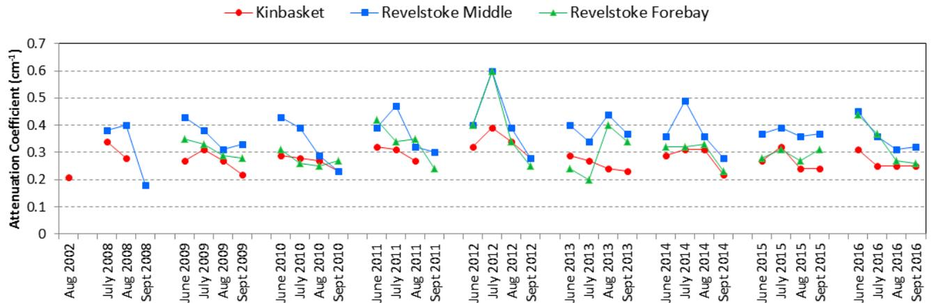
Figure 18. Attenuation coefficients ( $\text{cm}^{-1}$ ) in Kinbasket, Revelstoke Middle and Revelstoke Forebay from 2002-2016. Attenuation coefficients were calculated from Secchi disk depths in 2002 and 2008 and from the vertical profiles of photosynthetically available radiation in 2009-2016.
