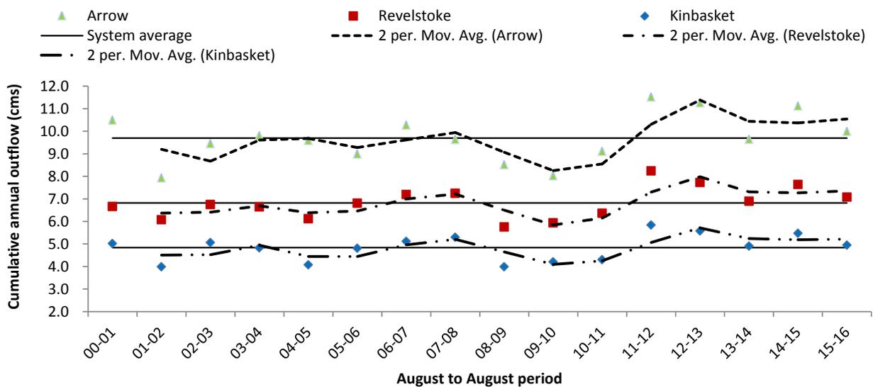
Figure 54. Cumulative outflow from August 1<sup>st</sup> to July 31<sup>st</sup> the following year for Kinbasket Reservoir (Mica Dam), Revelstoke Reservoir (Revelstoke Dam), and Arrow Reservoir (Hugh Keenleyside Dam) in millions of cubic metres per second.
