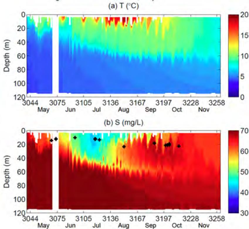
Figure 16. Contours of (a) temperature and (b) salinity from daily profiles collected using an autonomous profiler at Revelstoke Forebay, May to November 2016. (b) The '+' marks the 1% light level determined from Seabird profiles.
