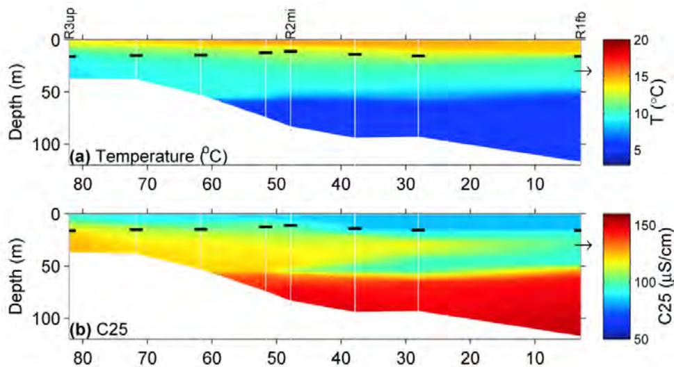
Figure 14. (a) Temperature and (b) conductivity (C25) in Revelstoke Reservoir, 8-9 September 2008. The inflow from Kinbasket Reservoir, which has slightly elevated conductivity, forms an interflow between 15 and 60 m depth which exits through the outlet marked by an arrow at 28 m on the right. White lines mark the location of the CTD casts. Black bars mark the depth of the photic zone.
