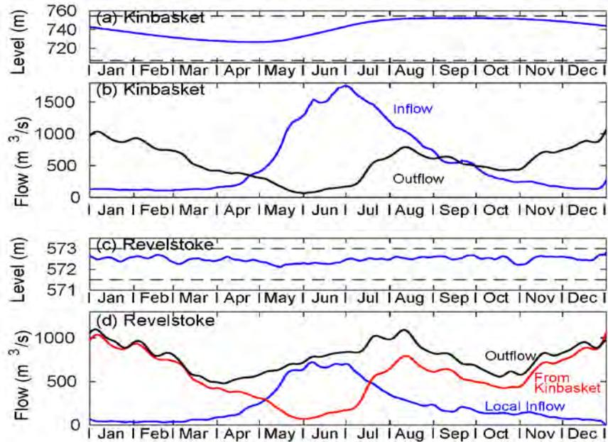
Figure 2. (a) Average water level for Kinbasket Reservoir, (b) average inflow and outflow for Kinbasket Reservoir, (c) average water level for Revelstoke Reservoir, and (d) average local inflow, inflow from Kinbasket Reservoir, and outflow for Revelstoke Reservoir. All data were averaged for 2008-2016.
