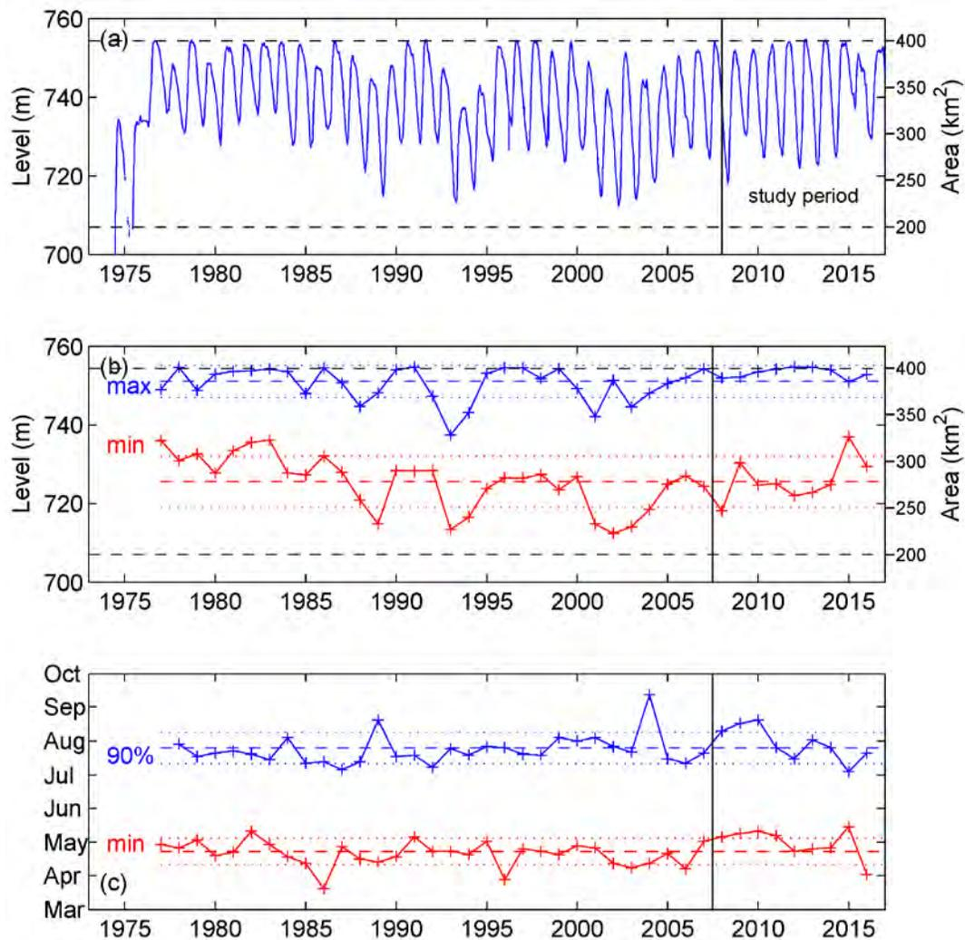
Figure 5. (a) Water level in Kinbasket Reservoir, 1973-2016. (b) Minimum (red) and maximum (blue) water level for 1977-2016. (c) Date of minimum (red), and 90% maximum (blue) water level for 1977-2016. The time to 90% full is shown as the time to the maximum water level can occur later in some years. Black dash lines mark normal minimum and maximum water level. Red and blue dash lines mark the average, and dotted lines mark  $\pm 1$  standard deviation.
