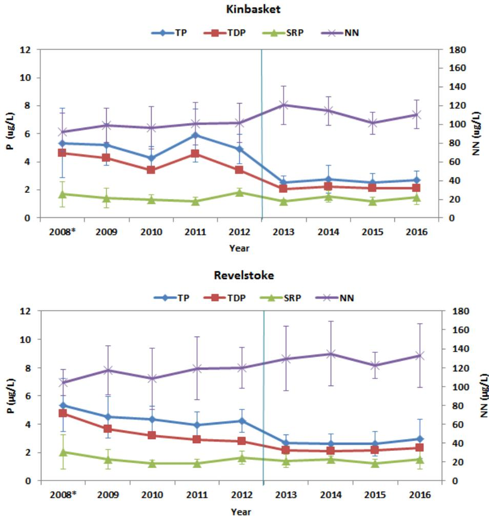
Figure 17. Average annual NN, TP, TDP, and SRP in Kinbasket and Revelstoke Reservoirs, 2008-2016. Error bars for are ±1 standard deviation and are not included for TDP (to keep the graph readable). Vertical blue line indicates when laboratory change occurred starting 2013. \*Note that the 2008 average is based on a partial year.
