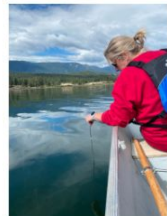
Volunteer, Ronda Ellery measuring water temperature, dissolved oxygen and conductivity.
