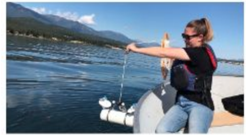
Program Coordinator, Georgia Peck using a Van Dorn to collect water samples from below the surface
