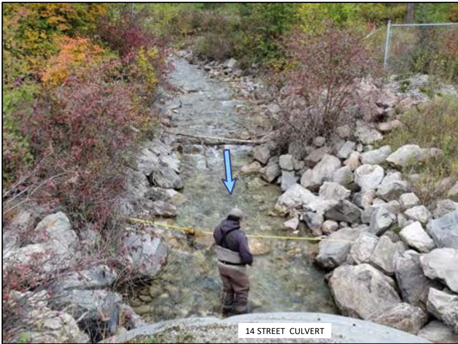
Photo 46 - September 28, 2019: Measuring flow upstream of the 14 Street culvert with an Acoustic Doppler Velocimeter.
