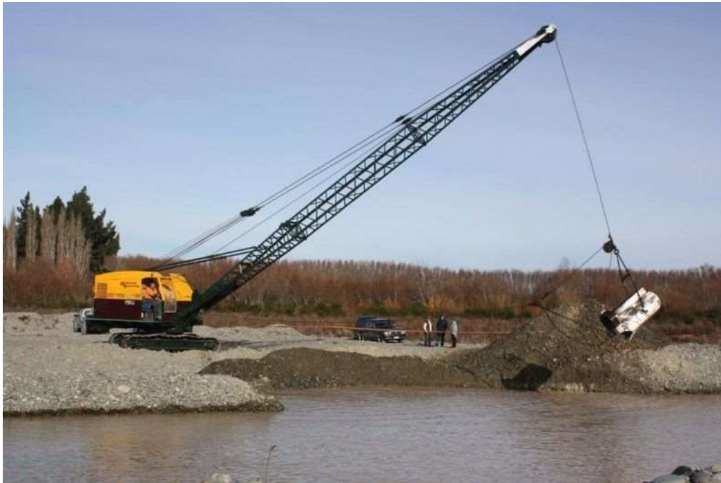
Figure 39. This photo shows a dragline working to move soil. Draglines were used to dig the ditches and build the dikes in Moberly Marsh.
