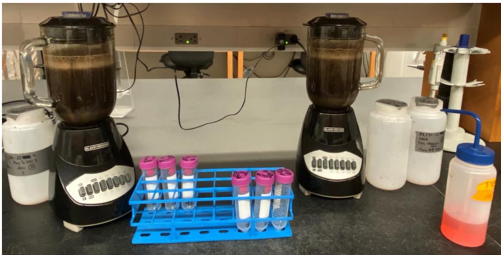
Figure 8: Sample homogenization of plant material, biota and sediment at the Hajibabaei laboratory in preparation for Next Generation Sequencing (NGS). Photo from STREAM (2023).
